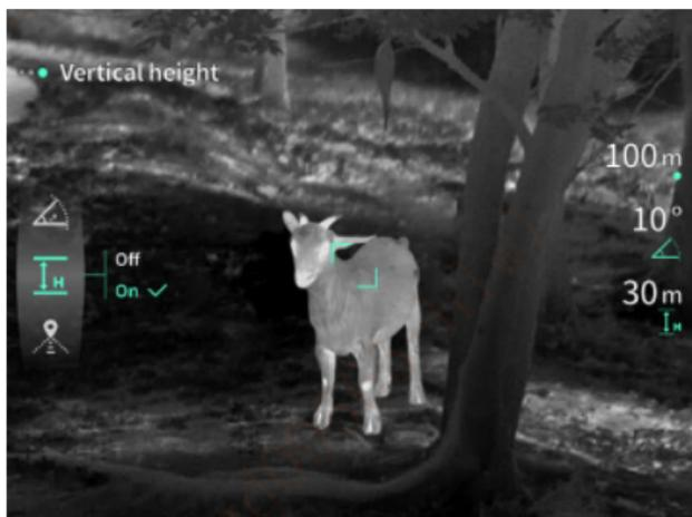
**Image enlargement:** the real-time image is electronically enlarged at the magnification of 1x, 2x, 4x and 8x by short pressing the Up button, and at the electronic magnification of 0.1x by long pressing the Up button.
